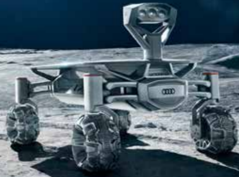
The Audi Lunar Quattro rover. An adjustable solar panel will capture sunlight and direct it to a lithium-ion battery, which will power four electric wheel hub motors. The vehicle's top speed is 3.6 kilometres per hour. Given the unevenness of the Moon's surface, the rover's off-road capabilities and ability to stay on course are vital. Three cameras will be mounted on the front: two stereoscopic and one scientific. The latter is for examining materials.
